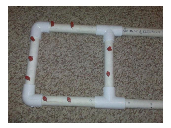
Once complete, use the remaining 6" pipe to connect the manifold to the pump via the adaptor. Be sure to use an equivalent pump as the Eco Plus 396 GPH pump was too small for this size manifold. I would not go below 600 GPH. Also, I was going to use a 1500 GPH sump pump from Menards for \$50, but those things use huge power; 500W vs 35W.
